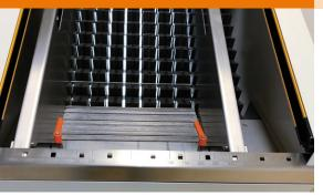
Max. filling quantity of bars with a length of 500mm
