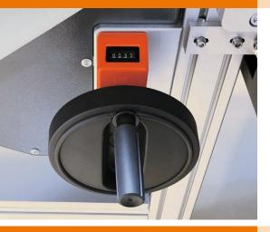
On the input loader the part diameter will be easily adjusted by using the mounted hand wheel.
