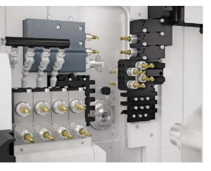
Standard to the Swiss GT 13 is a counter-operation station equipped with a Y axis that can house eight tools. Operations and counter-operations are performed completely independently of one another. Increasing your freedom of programming are this solution's spindle and counter spindles with identical power ratings, so you can say goodbye to the days of choosing heavy bar operations due to insufficient power in counter operations.
