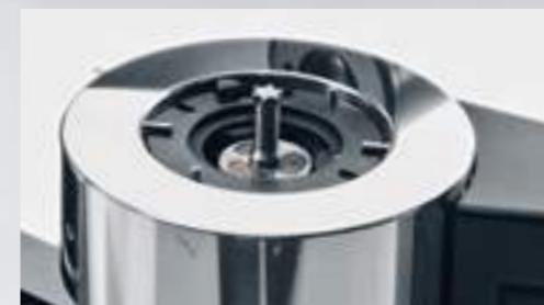
Fully automated with »tribos« The SCHUNK TRIBOS clamping unit is automatically positioned to the clamping position and returned to the starting position at the end of the clamping/ unclamping process.
