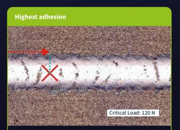
The high level of metal ionization ensures best adhesion. A scratch load of 120 Newtons for the Si-doped – and therefore very hard – InoxaCon<sup>®</sup>coating is extraordinary. The AlTiN-based product FerroCon<sup>®</sup> achieved up to 130 Newtons.
