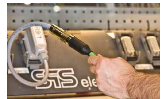
100% tested: digital continuity test
