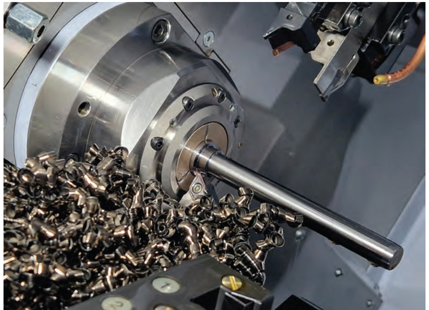
DunnAir on STAR SX38. Material : tooling steel Ø22mm, tolerance h9 cold drawn. Machining : one cutting pass with 2 simultaneous tools on Ø16mm. Goal : Finished Ø16x120mm with cylindricity less than 15 microns. Result with base guide bushing system : Parts cylindricity = 30 to 50microns Result with DunnAir guide bushing system : Parts cylindricity 5 to 10 microns
