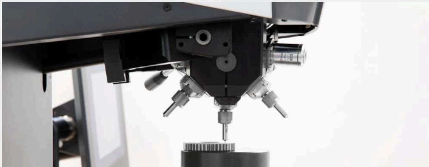
DUROMÈTRES BRINELL / KNOOP / ROCKWELL / VICKERS CS/C EVO
