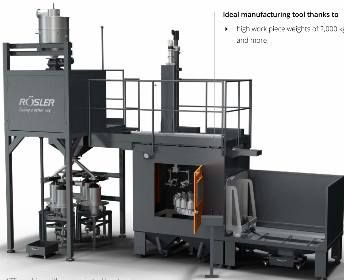
ATT machine with sophisticated blast system
