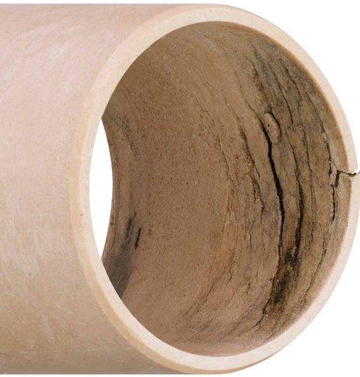
Damage due to permanent overload (Source: igus®)
