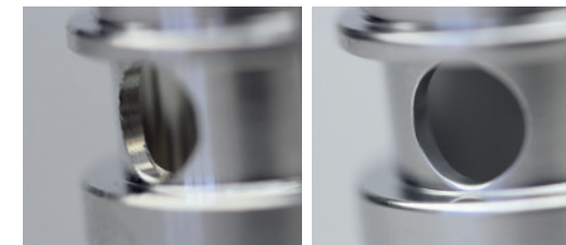
Example: before with burring, after completely free of burrs
