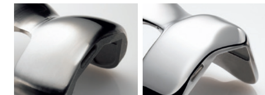
Example: highly polished surface, Ra 0.01 \mu m
