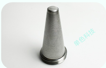
Filter Nozzle Drilling Material: 15-5PH CRES Aperture: \Phi 150\mu\text{m} \pm 1\mu\text{m} Wall Thickness: 0.5mm Field: Aerospace
