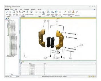
Leverage CAD product structures to dynamically generate parts lists with call outs and maintain associativity with engineering model to automate changes when product design changes occur.
